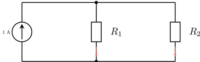
$$\frac{I_1}{I_2} = \frac{R_2}{R_1} \quad (3.11)$$
