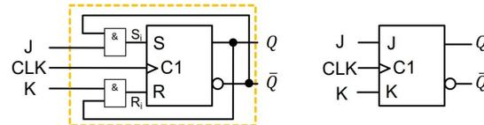
$$Q_{n+1} = (J \wedge \bar{Q}_n) \vee (\bar{K} \wedge Q_n) \quad \text{Wenn CLK } 0 \rightarrow 1$$
