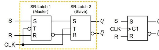
$$Q_{n+1} = [S \vee (Q_n \wedge \bar{R})]_n \quad \text{Reqs: } R \wedge S = 0, \text{ CLK } 0 \rightarrow 1$$
