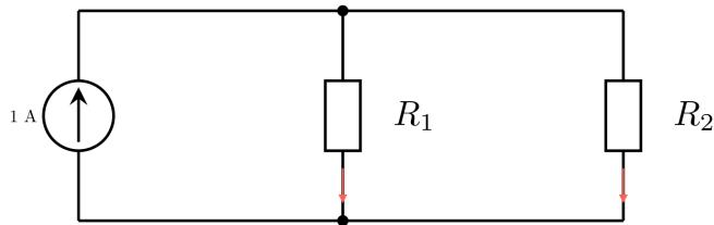
$$\frac{I_1}{I_2} = \frac{R_2}{R_1} \quad (3.11)$$
