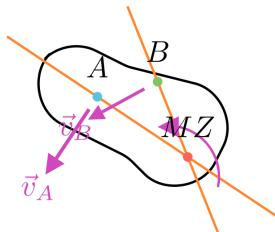
$$\vec{v}_A = \vec{v}_B + \vec{\omega} \times \vec{r}_{BA} \quad (1.7)$$
