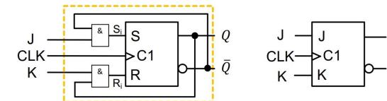
$$Q_{n+1} = (J \wedge \bar{Q}_n) \vee (\bar{K} \wedge Q_n) \text{ Wenn CLK } 0 \rightarrow 1$$
